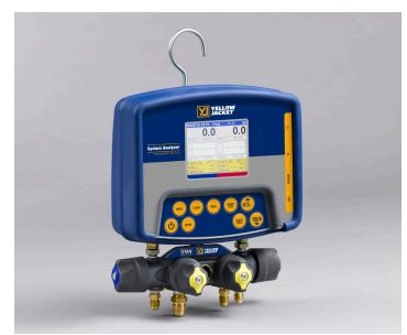
The YELLOW JACKET<sup>®</sup> Refrigeration System Analyzer (RSA) features a full color graphics display for intuitive, easy reading. The display reads in analog, digital or a combination of both, and monitors two pressures, two live temperatures, subcooling and superheat, and saturation temperatures (liquid and vapor) for nearly 100 NIST refrigerants.
