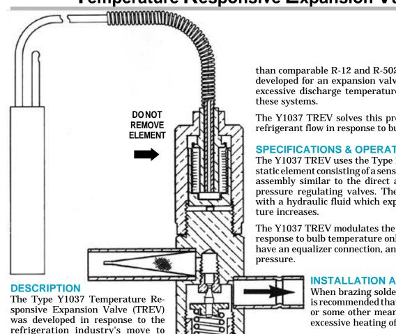
than comparable R-12 and R-502 systems, a need has developed for an expansion valve which will prevent excessive discharge temperatures from occurring on
