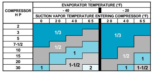
Selection based on R22, 100°F liquid and 10°F bulb temperature change \*For selections at conditions other than listed above see reverse side.
