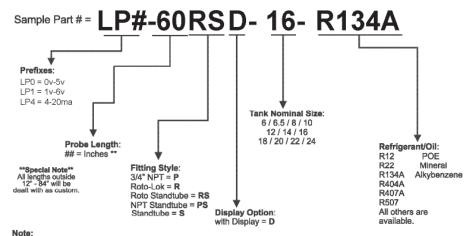
Stand-alone probes will come pre-adjusted for 0% and 100%. All other probes will have approximate settings for 0% & 100%. Ordering examples, LP-60P is a 60" probe with a 3/4" NPT connection; LP-60R is a 60" probe with Rotolock; LP-60RD is a 60" probe with both Rotolock and display options.
