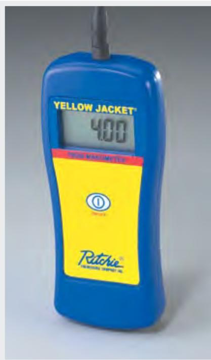
The digital electronic manometer eliminates the mess and fragility of U-tubes or diaphragm type gas pressure gauges. This easy-to-use instrument provides a continuous display of the measured positive or negative pressure. Ideal for setting gas pressure at manifold, checking pressure, flue draft and air balancing. Kit includes battery, 18" tubing and brass fitting.
