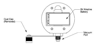
Rear View (Battery Cover Removed)
