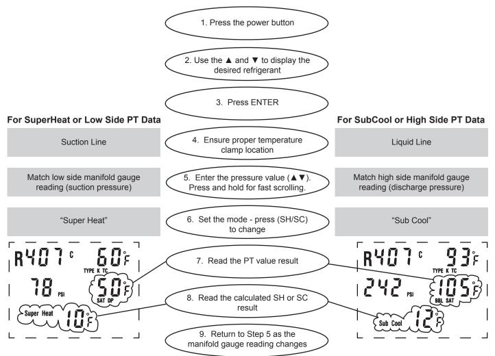
Note: The unit will not display a negative superheat or subool temperature. "--" will display instead. Make sure you have the proper temperature clamp location (Step 4) and the proper pressure value (Step 5).
